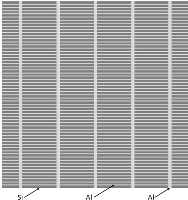
Fig. 4. Possible segmented Al pattern (gridlines feeding busbars).
