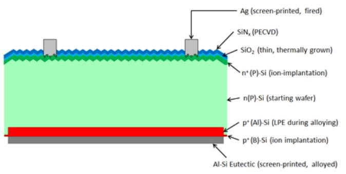
Fig. 1. Structure of Al alloy rear junction cell with extended emitter, as indicated by the short section labeled p<sup>+</sup>(B).
