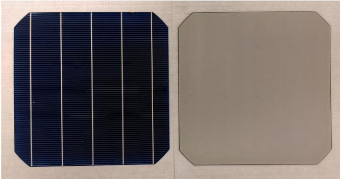
Fig. 2. Photograph of the front and back of an Al alloy rear junction cell with extended emitter (156 mm pseudosquare), fabricated according to the process of Table I.
